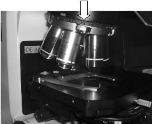
6.4 Verify that field is dark. Rotate polarizer for minimum transmission (normally when set to  $-o-$ )
