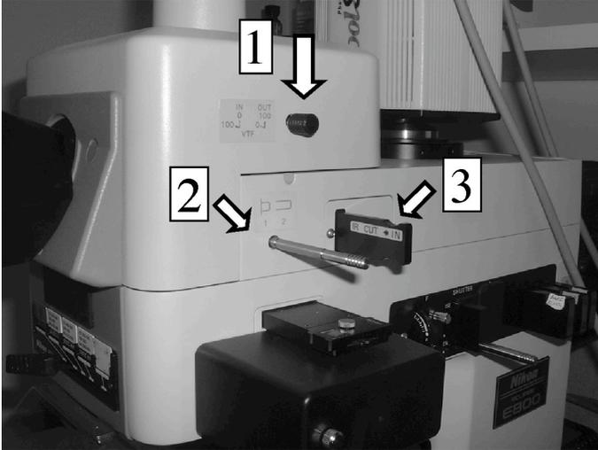
Lower Slider (2) IN: Coolsnap HQ High Resolution Monochrome CCD Camera
