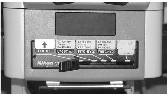
Filter positions (from left to right). [Note: Positions 1-4 are generally fixed. Position 5 may be occupied by a different filter (e.g. Texas Red or Cy5)]:
