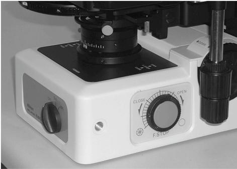
5.2 Focus field diaphragm by moving condenser UP or DOWN (1)
