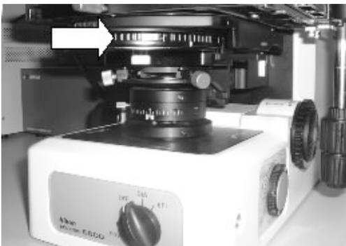
6.3 Disengage objective prism by pulling prism slider OUT (without removing completely; the DIC objective prisms are the little sliders located just above each objective). Note: make sure to disengage the prism directly above the objective in use (in the image below, the prism shown belongs to an objective that is NOT in use).
