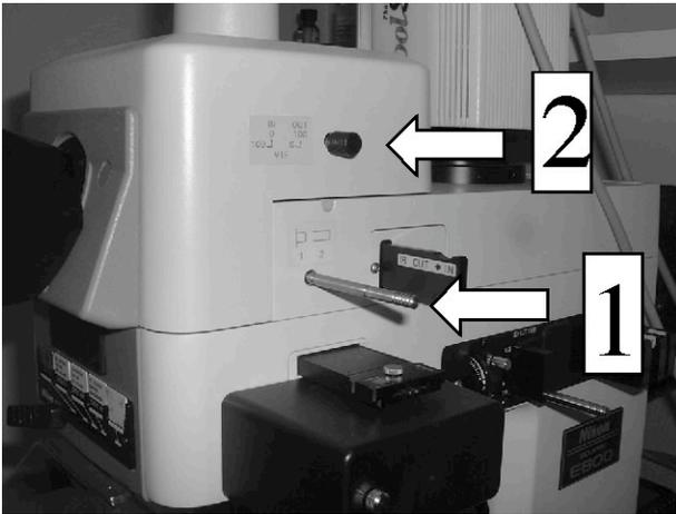
Lower Slider (1) IN: Coolsnap HQ High Resolution Monochrome CCD Camera
