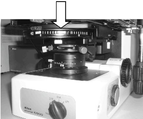
As an approximation, the condenser aperture should be set to minimum for 10x objective and to max for 100x objective:
