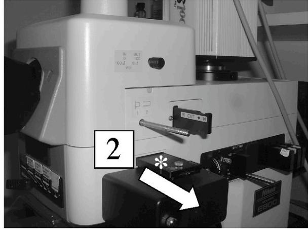
3.9. Set Condenser turret to position A (for normal transmitted light)
