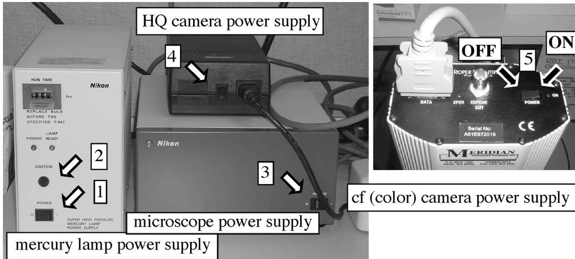
2.1 Power ON Mercury (Hg) arc lamp (if using fluorescence).
