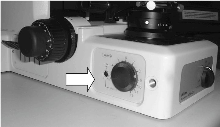
3.7. Engage filters for transmitted illumination if required (e.g. neutral density to attenuate light). Push lever down to engage filter.
