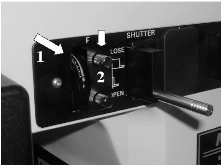
7.7 Always pull shutter OUT when not imaging or viewing to minimize photobleaching of your sample.
