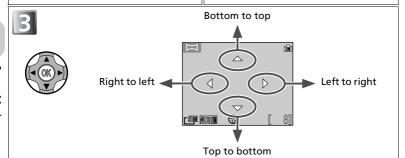
Select how pictures will be joined together in completed panorama. This is the direction in which to pan the camera after each shot.
