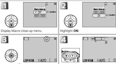
Exit menu. icon appears in monitor when camera is in Macro close-up (to exit without setting Macro close-up mode, wait two seconds without pressing Button).
