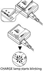
CHARGE lamp starts blinking when battery is inserted. Charging is complete when lamp stops blinking.
