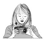
When the shutter-release button is pressed half way, the camera will automatically adjust focus according to the distance to the subject. If the focus operation is successful, the AF(Autofocus)/ Flash indicator next to the viewfinder will glow green. The focus setting will remain unchanged as long as the shutter button is half-pressed (see the section "Focus Lock" in the *Fast Track Guide*). The zoom ratio for digital zoom cannot be changed while focus lock is in effect.
