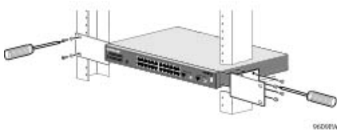
Figure 3-1. Attaching Mounting Brackets
