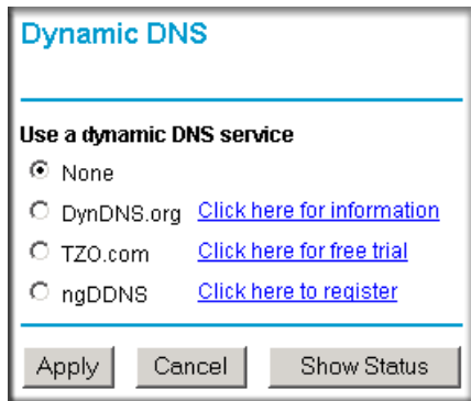
Figure C-8: Dynamic DNS Setup Screen
