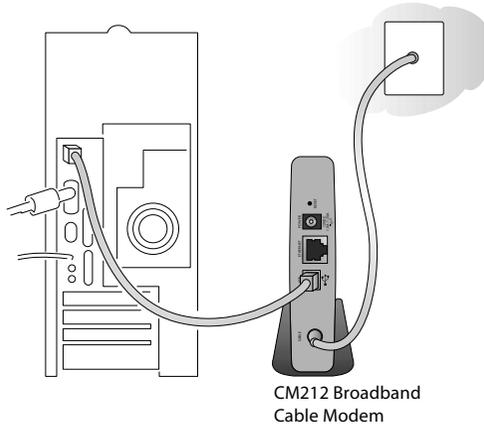
Once the Modem establishes a link with your service provider, the PC will automatically detect the modem on the USB port.
