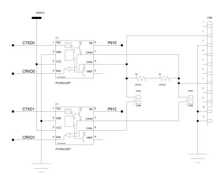
Figure 5: CAN transceivers
