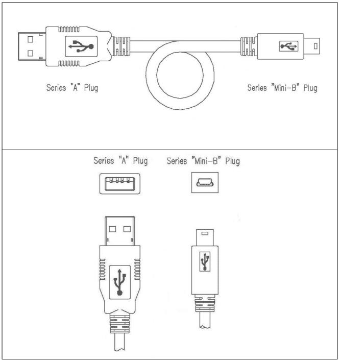
Figure 70: USB interface cable (Mini-B type)
