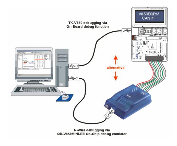
Figure 6: Configuration for On-Chip debugging
