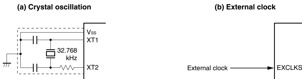
Figure 5-10. Example of External Circuit of XT1 Oscillator (Crystal Oscillation)
