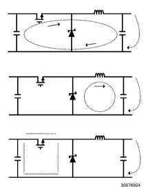
FIGURE 3. Current Flow in a Buck Application
