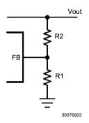
FIGURE 2. Resistive Feedback Divider
