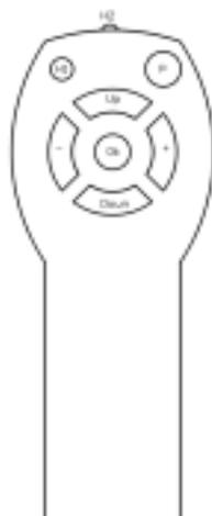
After exchanging the cells the IR06 needs to be programmed to the MMIB specific device code (166). Therefore press [P] and [OK] together until the red LED (H1) is permanent on. Then press in following order:
