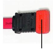
Take out the dust cover and connect to the hard disk devices
