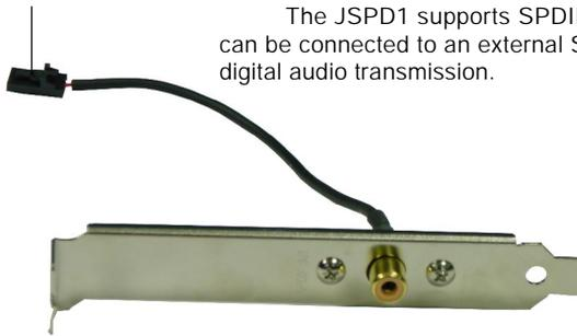
The JSPD1 supports SPDIF output only and can be connected to an external SPDIF Bracket for digital audio transmission.
