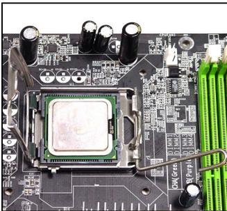
8. Rotate the load plate onto the package.
