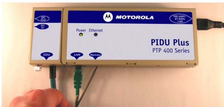
Figure 4 - PTP 400 Series Bridge Recovery Switch Location
