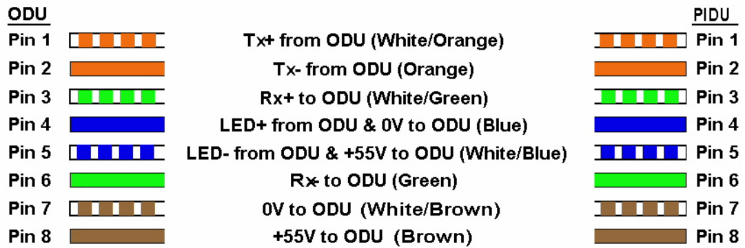
Figure 75 - ODU to PIDU Plus Connection Diagram
