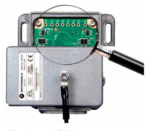
Figure 106 - PTP LPU Test Points
