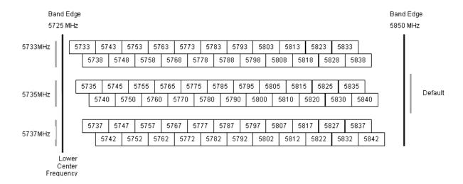
Figure 130 – PTP 58500 Available Spectrum Settings – 5 MHz Channel Bandwidth
