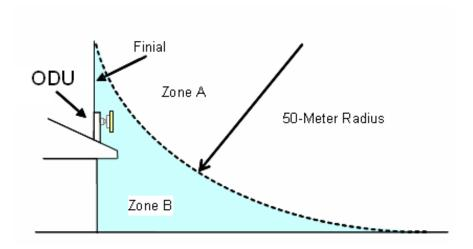
In Zone B, a direct lightning strike is unusual, but the un-attenuated electromagnetic field is still present. Equipment mounted in Zone B should be grounded using grounding wire of at least 10 AWG. This grounding wire should be connected to a grounding rod or the building grounding system before entry in to building.
