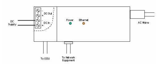
Figure 8 - External DC Supply and Redundant AC Supply
