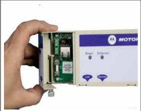
Step 1: Undo the retaining screw and hinge back the cover.
