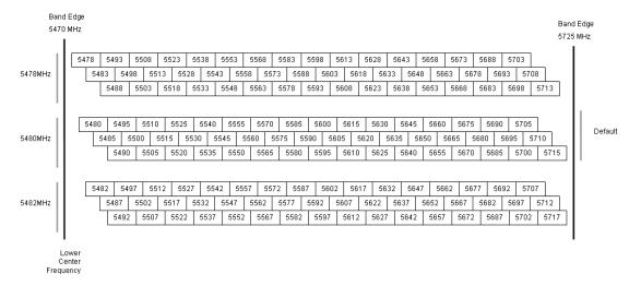
Figure 127 - PTP 54500 Available Spectrum Settings - 5 MHz Channel Bandwidth
