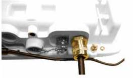
Step 4: Screw on the clamping nut and tighten (Do not over tighten – see Figure 25)
