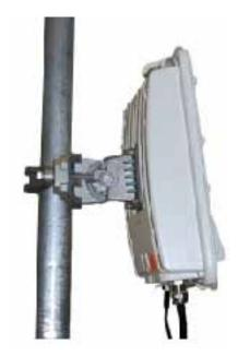
3. Adjust the elevation and azimuth of the unit before tightening to the required torque settings of 14 Nm (11 lb ft) for both bolts.
