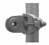
2. Offer the ODU (with pre-fitted mounting bracket) to the bracket strap and affix using the captive M8 bolt. Tighten to ensure the assembly grips, but can be adjusted on the pole (Figure 20 and Figure 21).
