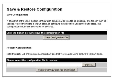
The configuration file format is **MAC-mm-mm\_IP-iii-iii-iii-iii.cfg**, where **mm** and **iii** are the lower 3 bytes of the MAC address and the unit IP address respectively.
