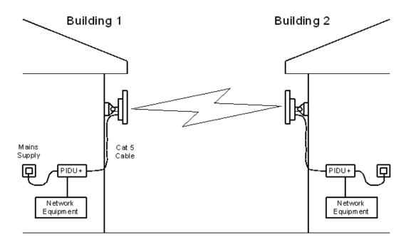
Figure 1 - Typical PTP 500 Series Bridge Deployment
