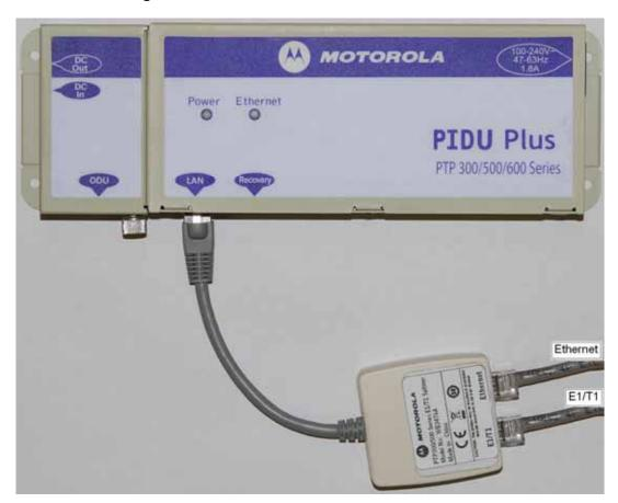
Figure 119 - PIDU Plus and E1/T1 Connexion
