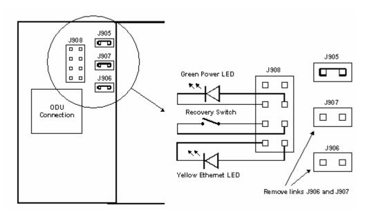
Figure 9 - Remote LED and Recovery Switch Wiring
