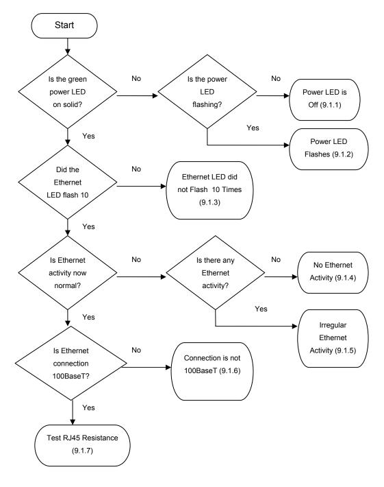
Figure 105 - Link End Hardware Test Flowchart
