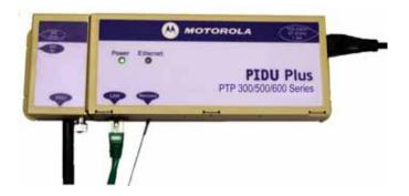
The Recovery switch is used to recover the unit from configuration errors or software image corruption. To put an ODU into recovery mode, the Recovery switch should be pressed, then the power applied. The Recovery switch should be kept pressed for at least 30 seconds after the power has been applied. Full instruction on the recovery mode can be found in Section 8 "Recovery Mode".
