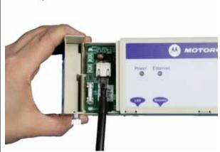
Step 2: Plug in the ODU into the PIDU Plus Cable ensuring that it snaps home.
