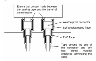
Figure 114 - Weatherproofing the Antenna Connections
