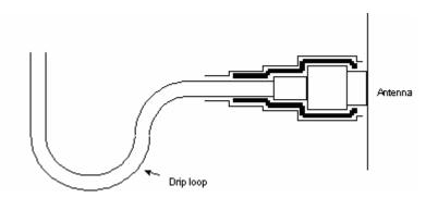
Figure 113 - Forming a Drip Loop
