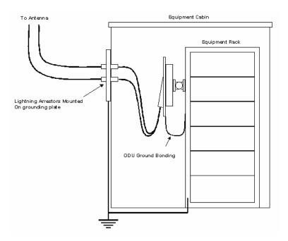
**Figure 116 - Lightning Arrestor Mounting**
