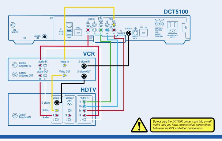
This diagram should be used if you intend to use a standard stereo VCR in your configuration. This configuration will allow you to watch both HD and Standard Definition video on your HDTV as well as record and play Standard Definition video via your VCR.
