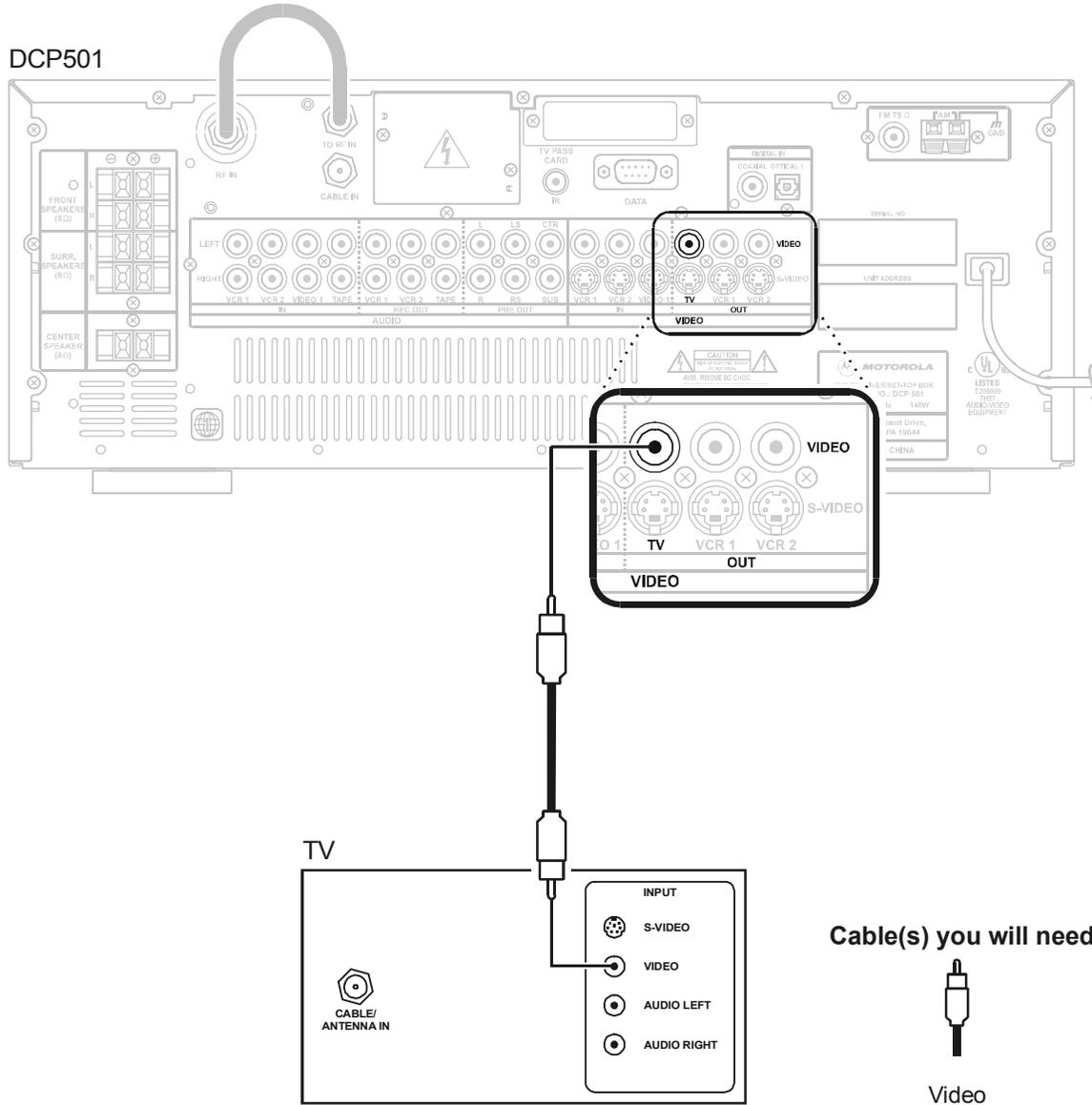
*When connecting the video path, never connect composite video and S-Video together. Because certain types of electronics equipment will not support both video inputs simultaneously, use only one connection path.*
