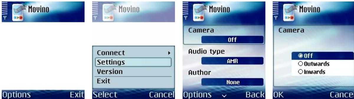
Video and audio can be streamed either to the Movino OS X desktop client via Bluetooth or a Movino video server via TCP/IP. This is selected from the *Connect* menu. More detailed information regarding connecting is found in the *Connect* section.
