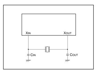
Fig. 40 External circuit of ceramic resonator
