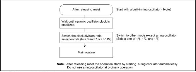
Fig. 6 Switching method of CPU mode register
