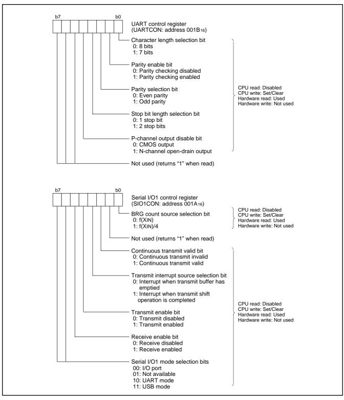
Fig. 28 Structure of serial I/O1-related registers (5)
