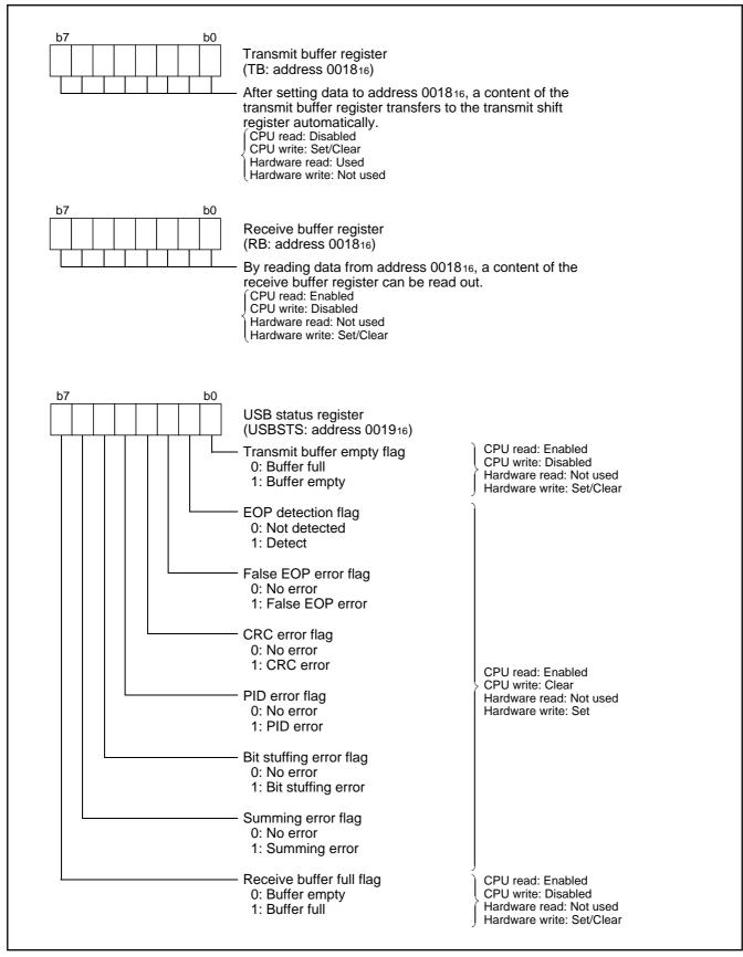
Fig. 24 Structure of serial I/O1-related registers (1)
