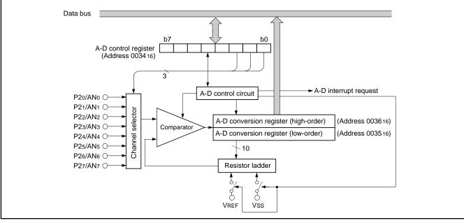
Fig. 34 Block diagram of A-D converter
