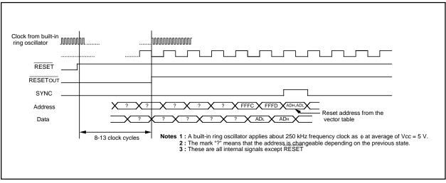
Fig. 38 Timing diagram at reset
