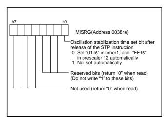
Fig. 42 Structure of MISRG
