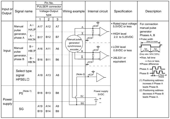
(Note-1): The 5V(P5)DC power supply from the Q173PX must not be connected if a separated power supply is used as the Manual pulse generator/Incremental synchronous encoder power supply. Use a 5V stabilized power supply as a separated power supply. Any other power supply may cause a failure.
