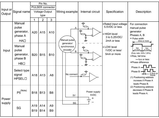
(Note) : The 5V(P5)DC power supply from the Q173PX must not be connected if a separated power supply is used as the Manual pulse generator/Incremental synchronous encoder power supply.
