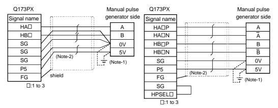
(Note-1): The 5VDC(P5) power supply from the Q173PX must not be connected if a separate power supply is used as the Manual pulse generator/Incremental synchronous encoder power supply.
