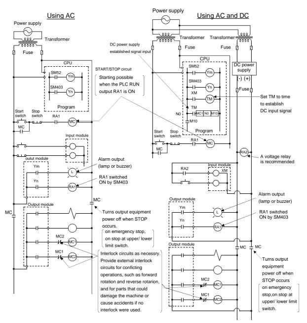
The power-ON procedure is as follows: For AC
