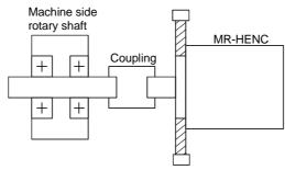
Fig 4.2 Connecting the encoder to a machine side rotary shaft.
