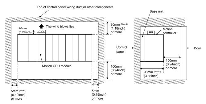
(Note-1): 20mm (0.79 inch) or more when the adjacent module is removed and the extension cable is connected.
