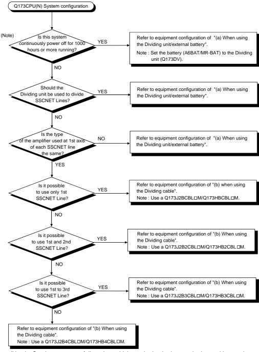
(Note): Continuous power failure time which can be backed up on the internal battery is different depending on the charge time. It is possible to continuously power off for 1100 hours because of charge of 40 hours. Refer to the section 2.3(5) for details.
