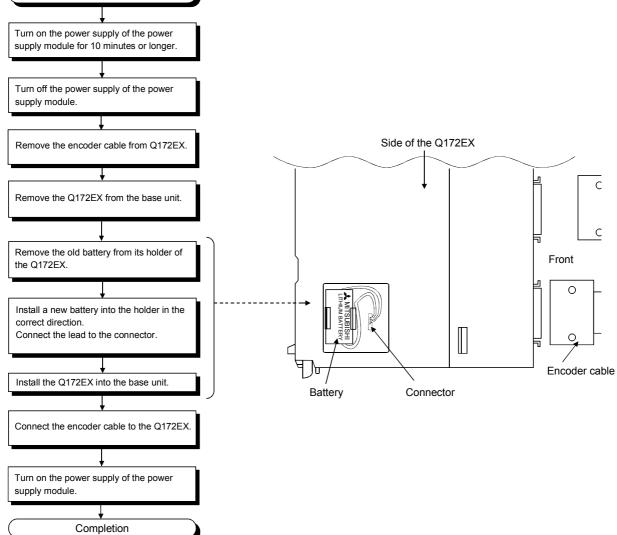
(2) Battery replacement procedure of the Dividing unit, Battery unit When the battery has been exhausted, replace the battery with a new one in accordance with the procedure shown below.
