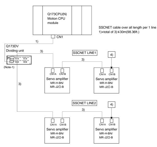
(Note-1): When using the external battery, set the Battery (A6BAT/MR-BAT) into the Dividing unit (Q173DV).
