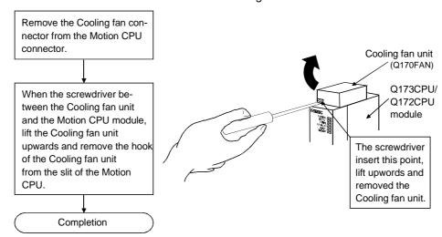
(b) Installation of Cooling fan unit on Q173CPU/Q172CPU The installation of the Cooling fan unit are described below.
