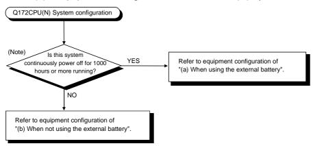
(Note): Continuous power off time which can be backed up on the internal battery is different depending on the charge time. It is possible to continuously power off for 1100 hours because of charge of 40 hours. Refer to the section 2.3 (5) for details.
