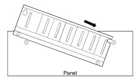
3) Place the left-hand side pear-shaped hole of the CPU base unit onto the left-hand side screw.
