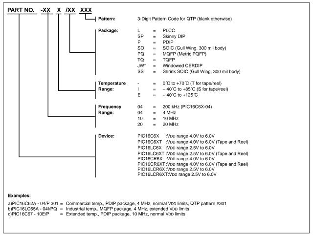
\* JW Devices are UV erasable and can be programmed to any device configuration. JW Devices meet the electrical requirement of each oscillator type (including LC devices).
