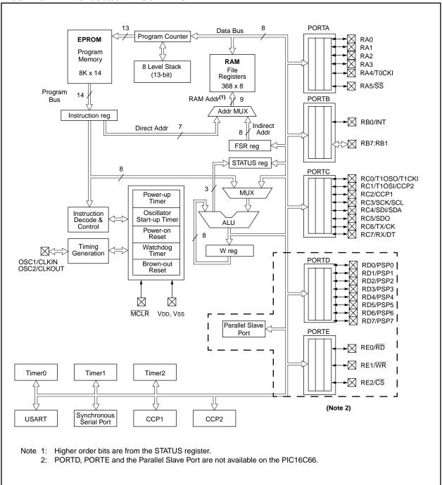
FIGURE 3-4: PIC16C66/67 BLOCK DIAGRAM
