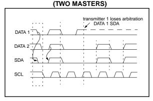
Masters that also incorporate the slave function, and have lost arbitration must immediately switch over to slave-receiver mode. This is because the winning master-transmitter may be addressing it.
