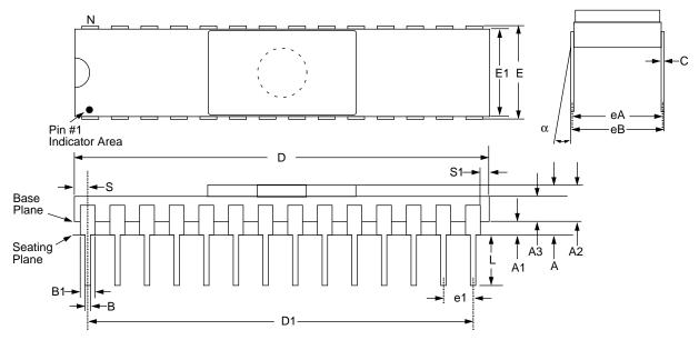
25.9 28-Lead Ceramic Side Brazed Dual In-Line with Window (300 mil) (JW)
