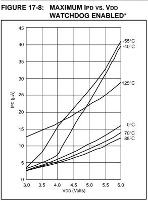
\*IPD, with Watchdog Timer enabled, has two components: The leakage current which increases with higher temperature and the operating current of the Watchdog Timer logic which increases with lower temperature. At -40°C, the latter dominates explaining the apparently anomalous behavior.
