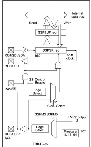
To enable the serial port, SSP enable bit SSPEN (SSPCON<5>) must be set. To reset or reconfigure SPI mode, clear enable bit SSPEN, re-initialize SSPCON register, and then set enable bit SSPEN. This configures the SDI, SDO, SCK, and SS pins as serial port pins. For the pins to behave as the serial port function, they must have their data direction bits (in the TRIS register) appropriately programmed. That is:
