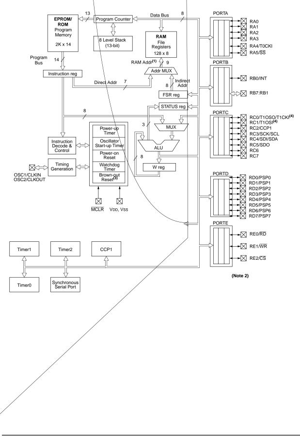
FIGURE 3-2: PIC16C62/62A/R62/64/64A/R64 BLOCK DIAGRAM
