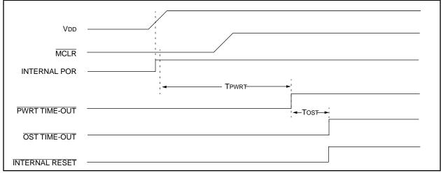
FIGURE 13-12: TIME-OUT SEQUENCE ON POWER-UP (MCLR NOT TIED TO VDD): CASE 2
