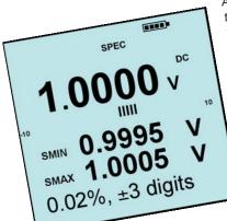
Another innovative feature is the instrument's **SPEC** function, which automatically displays measurement tolerances without the user needing to calculate it.
