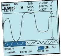
The **MEM** function enables you to record up to 6500 date/time measurements, for periods ranging from 1 sec to 24 hrs, and to analyse the results graphically for up to 4 simultaneous measurements.
