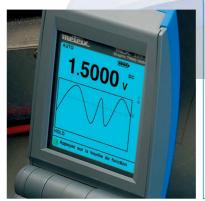
Selected modes and functions, as well as physical and electrical values, and relevant warning symbols, are all clearly displayed on the instrument's160 x 160 highresolution graphic display.
