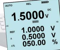
Thanks to the instrument's 4 digital displays, the relative function **REL** provides comprehensive simultaneous display of the absolute and absolute drift values, relative drift % and reference value. For greater comfort, the reference value can be adjusted directly using the **REL** function key.
