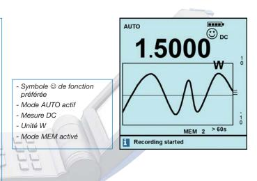
Thanks to technological improvements resulting in a single "A" terminal, current measurements may be carried out from a single switch position, making for fluid and trouble-free changes of the measurement range, from just a few hundred microamperes to up to 20 amperes.
