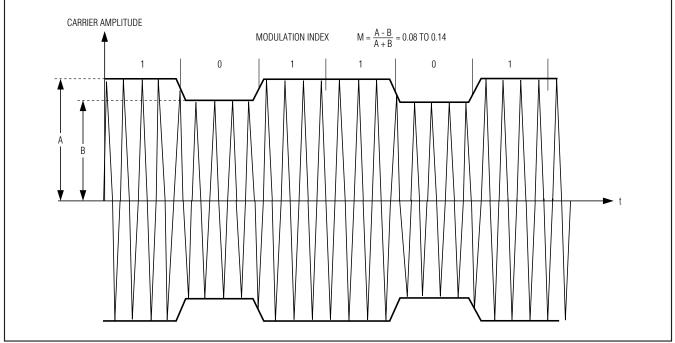
Figure 8. Downlink: 8% to 14% Amplitude Modulation
