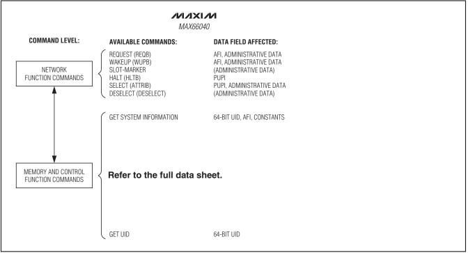
Figure 2. Hierarchical Structure of ISO/IEC 14443 Type B Protocol
