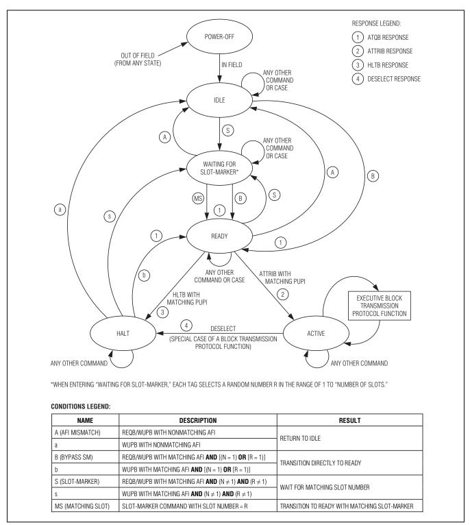
Figure 17. ISO/IEC 14443 Type B State Transitions Diagram
