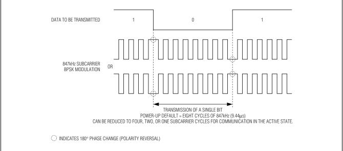
Figure 9. Uplink: BPSK Modulation of the 847.5kHz Subcarrier
