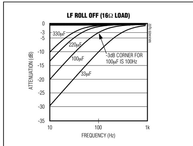
Figure 2. Low-Frequency Attenuation for Common DC-Blocking Capacitor Values
