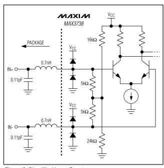
Figure 6. Simplified Input Structure
