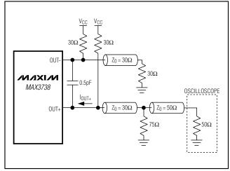
Figure 2. Test Circuit for Characterization
