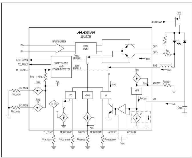
Figure 4. Functional Diagram
