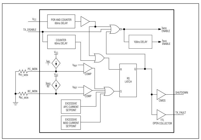
Figure 5. Simplified Safety Circuit
