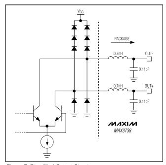
Figure 7. Simplified Output Structure
