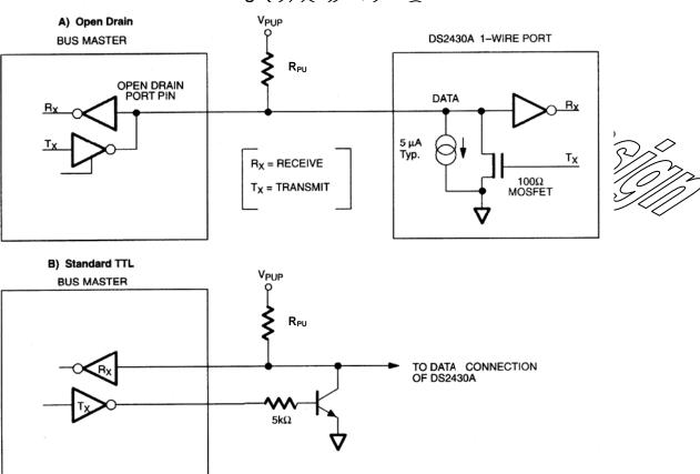
Note: Depending on the 1-Wire communication speed and the bus characteristics, the optimal pullup resistor value will be in the  $1.5k\Omega$  to  $5k\Omega$  range. To write to a single device, a  $2.2k\Omega$  resistor and  $V_{PUP}$  of at least 4.0V is sufficient. For writing multiple DS2430As simultaneously or operation at low  $V_{PUP}$ , the resistor should be bypassed by a low-impedance pullup to  $V_{PUP}$  while the device copies the scratchpad to EEPROM.
