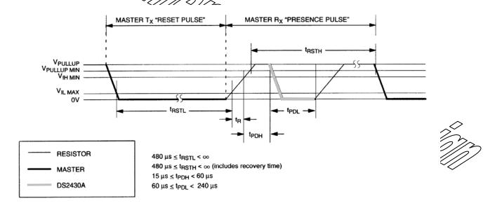
In order not to mask interrupt signaling by other devices on the 1-Wire bus,  $t_{RSTL} + t_R$  should always be less than 960 $\mu$ s.
