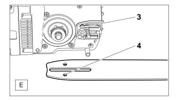
To guarantee a troublefree operation of the oil pump the oil guide groove (E/3) as well as the oil inlet bore in the guide bar (E/4) must be cleaned in regular intervals.
