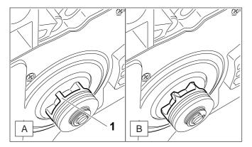
Check the sprocket (A/1) before mounting a new chain.
