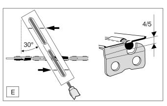
The file holder makes file guidance easier. It is marked for the correct 30° sharpening angle (keep the marks parallel with the chain when filing, see illustration) and limits the cut depth to the correct 4/5 of the file diameter. See "Accessories" for the order number.
