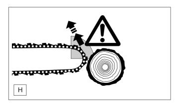
The UC 3001A, UC 3501A and UC 4001A comes with an inertial chain brake as standard equipment. If kickback occurs due to contact of the guide-bar tip with wood (see SAFETY PRECAUTIONS, page 7), the chain brake will stop the chain through inertia if the kickback is sufficiently strong.
