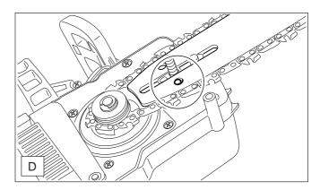
Position the guide bar. Take care that the pivot (A/4) of the chain tightener is inserted into the bore (see circle) of the guide bar.
