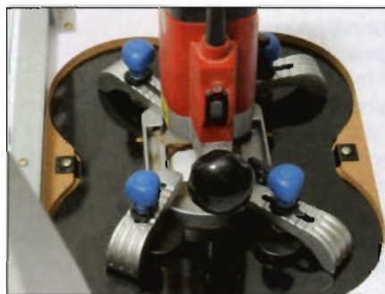
The quick and accurate clamping system
