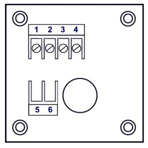
The base plate of the S model should be installed with terminals 1 to 4 placed on top. Preferably, use a cable with 18 AWG wires. Avoid running the cables connecting the unit in the same conduit as 110 VAC power cables. Depending on the installation, you may have to use a cable with twisted pairs or a shielded cable to avoid electromagnetic interference.
