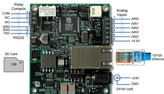
The MDL-IDM ships as a software-customizable module with the following features:
