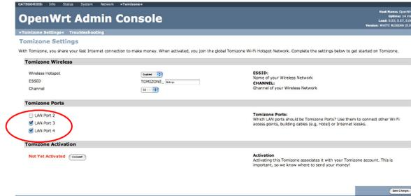
In this screen shot, you can see LAN Port 3 & 4 have been activated as Tomizone Ports. CONFIRM CHANGES BY CLICKING THE “SAVE CHANGES” button then “**APPLY CHANGES**” button – Now click on the “**Activate**” button, which will allow you to assign this router to your Tomizone account.
