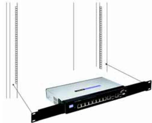
Figure 3-3: Mount the Switch in the Rack
