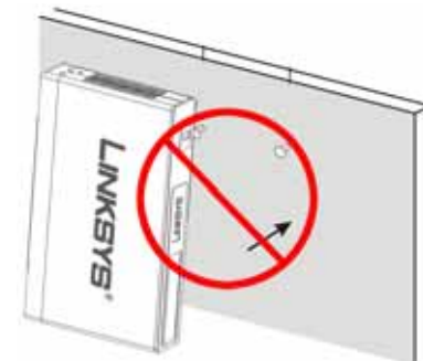
Figure 3-5: Incorrect Wall-Mount Orientation (Vertical)
