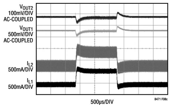
Figure 8c. Load Step on V<sub>OUT1</sub> from 40mA to 135mA to 40mA
