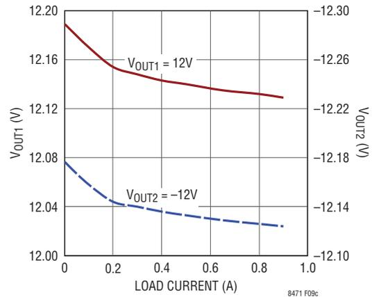
Figure 9c. 12V and -12V Outputs vs Load Current
