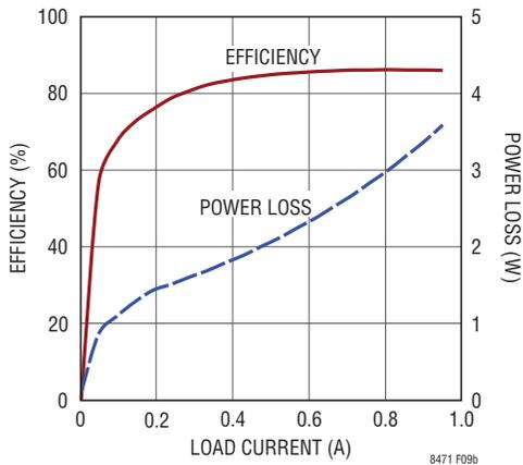
Figure 9b. Efficiency and Power Loss
