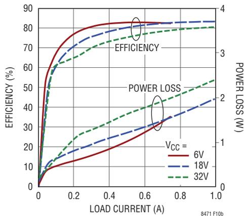
Figure 10b. Efficiency and Power Loss (Load from  $V_{OUT1}$  to  $V_{OUT2}$ )
