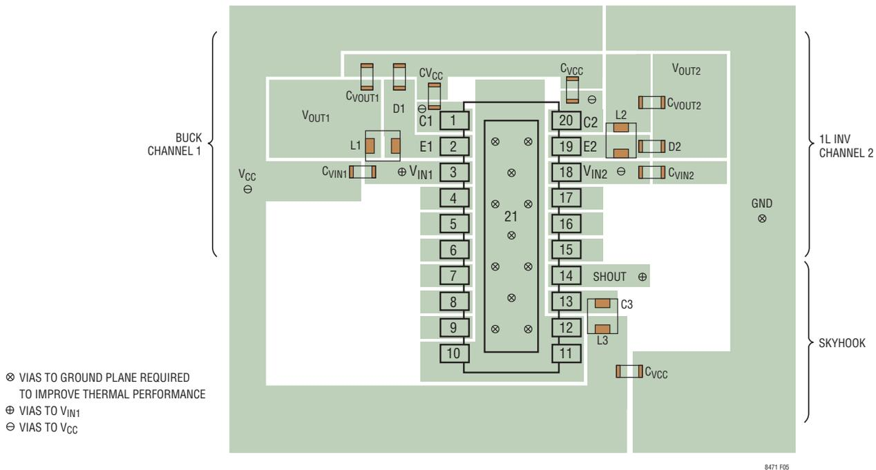
Figure 5. Suggested Component Placement for a Buck and Single-Inductor Inverting Converter
