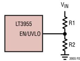
Figure 1. Resistor Connection to Set V<sub>IN</sub> Undervoltage Shutdown Threshold
