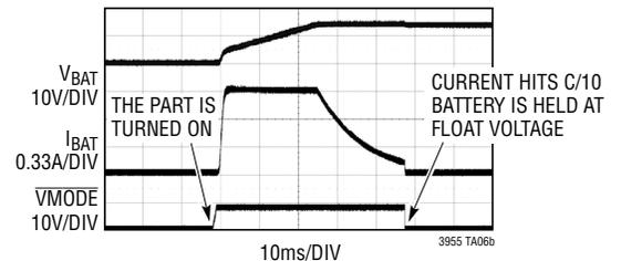
NOTE: WAVEFORMS SHOWN AS TESTED WITH 5Ω IN SERIES WITH 2mF CAPACITIVE LOAD.
