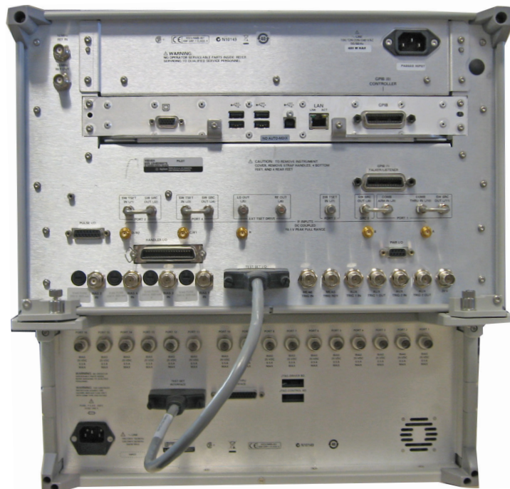
Figure 18 N5242A Test Set I/O Cable Connection
