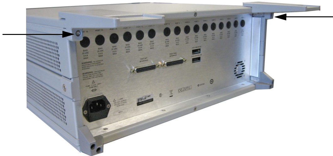
Figure 14 Install Locking Feet on U3042AE08
