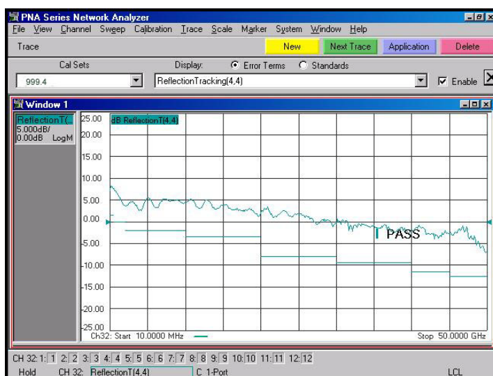
Figure 36 Reflection Tracking Trace (Port 1-12)
