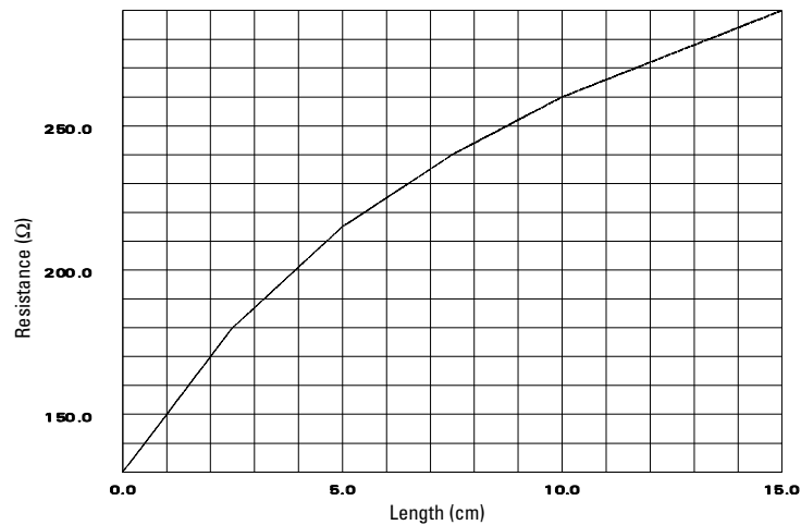
Optimum Damping Resistor Value Versus Signal Lead Length
