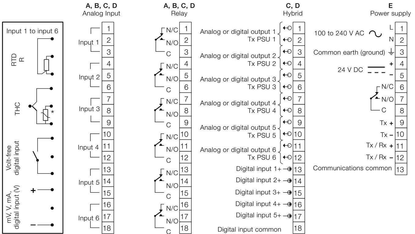
\* Each thermocouple input must have either a cold junction assembly (part number CM30/0052) or shorting link (part number RVG200/0118) fitted. Each analog input card with a thermocouple input must have a minimum of 1 cold junction assembly fitted. For applications requiring maximum thermocouple accuracy, it is recommended that each thermocouple input is fitted with a cold junction assembly.
