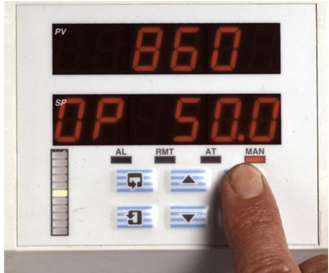
The clearly-labelled tactile keypad gives direct access for operator adjustments and configuration programming, without the need to open the recorder's door. Clear text prompts on the digital displays guide the user around the various menus. A password-protected security system prevents unauthorized access to configuration adjustment menus.
