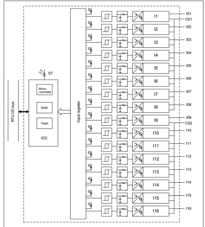
Figure 1: Block diagram 520BID01
