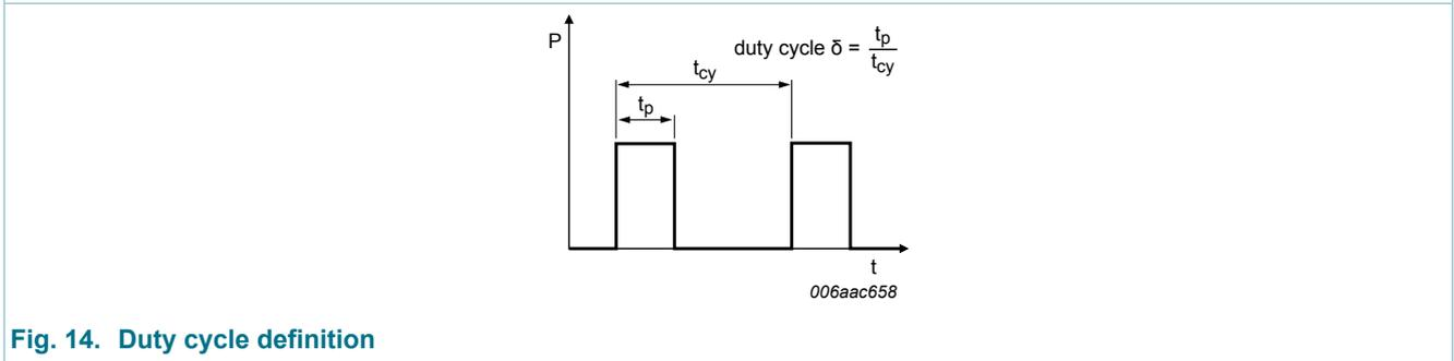
Fig. 14. Duty cycle definition
