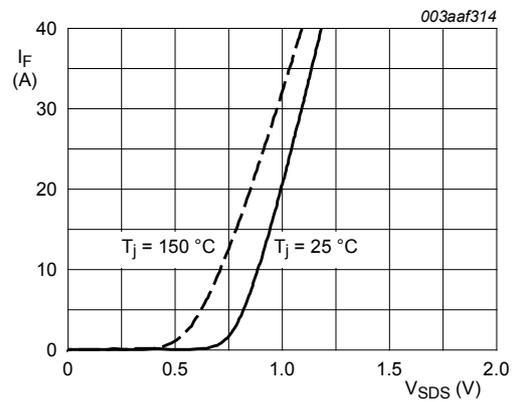
$V_{GS} = 0\text{ V}$
