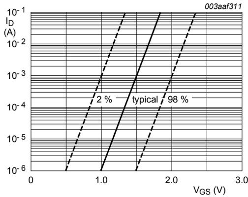
$T_j = 25\text{ }^\circ\text{C}; V_{DS} = V_{GS}$
