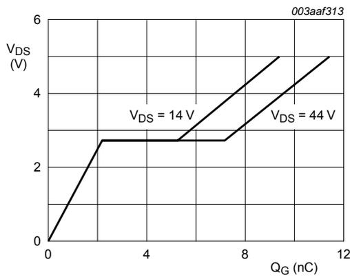
$T_j = 25\text{ }^\circ\text{C}; I_D = 7\text{ A}$
