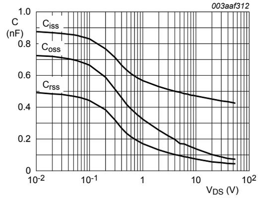
$V_{GS} = 0\text{ V}; f = 1\text{ MHz}$
