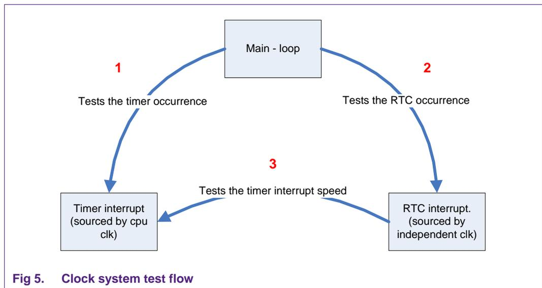
The second function is intended to be called from a timer interrupt service handler. This Timer needs to have the same clock source as the CPU.
