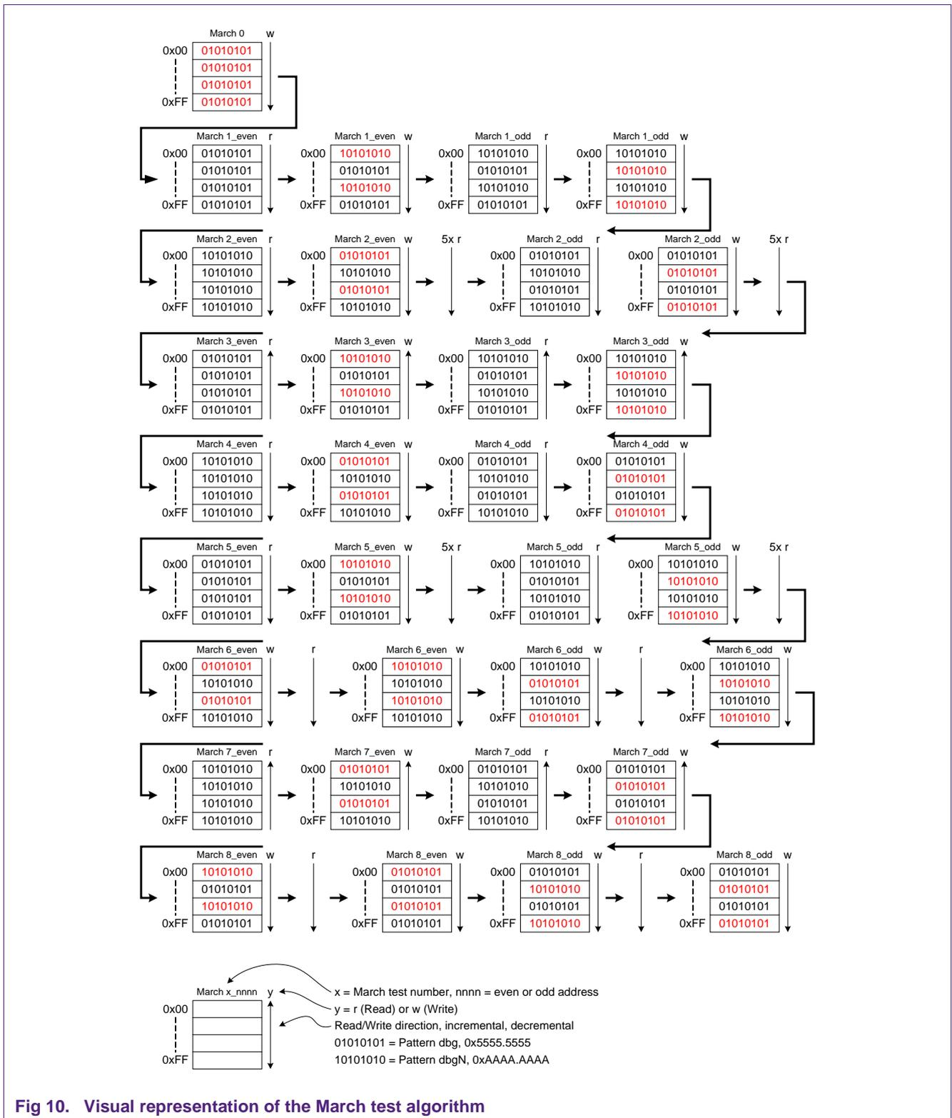
Fig 10. Visual representation of the March test algorithm
