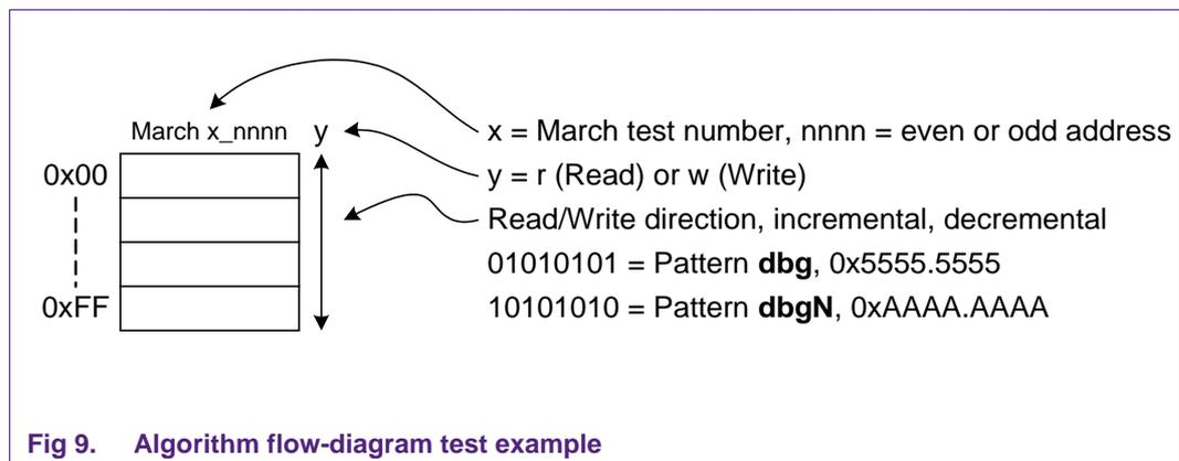
Fig 9. Algorithm flow-diagram test example
