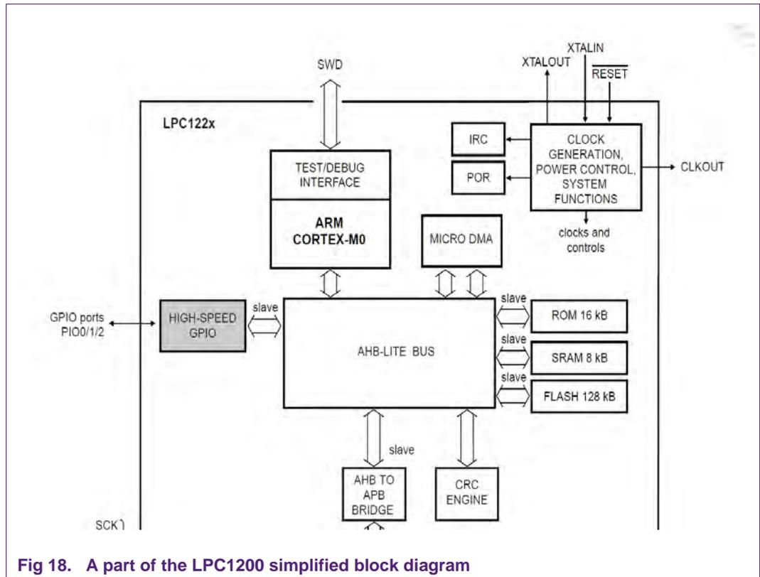
Fig 18. A part of the LPC1200 simplified block diagram
