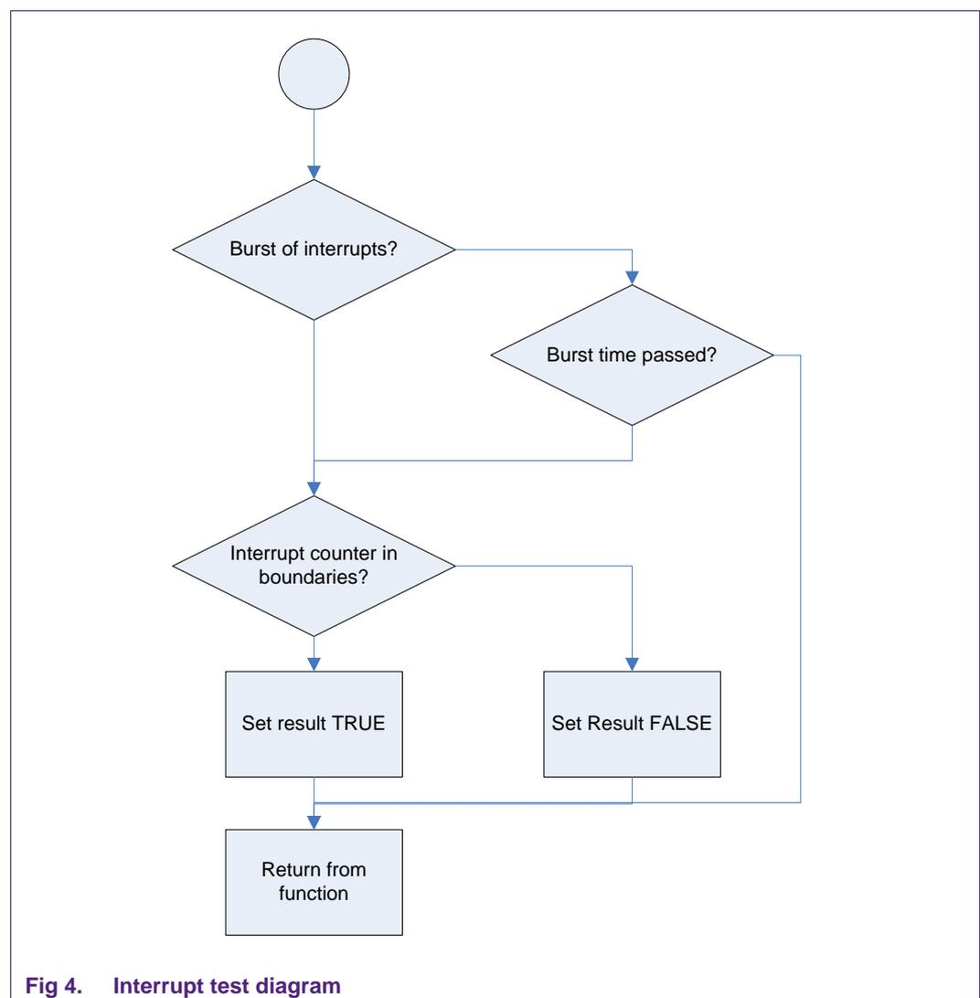
Fig 4. Interrupt test diagram
