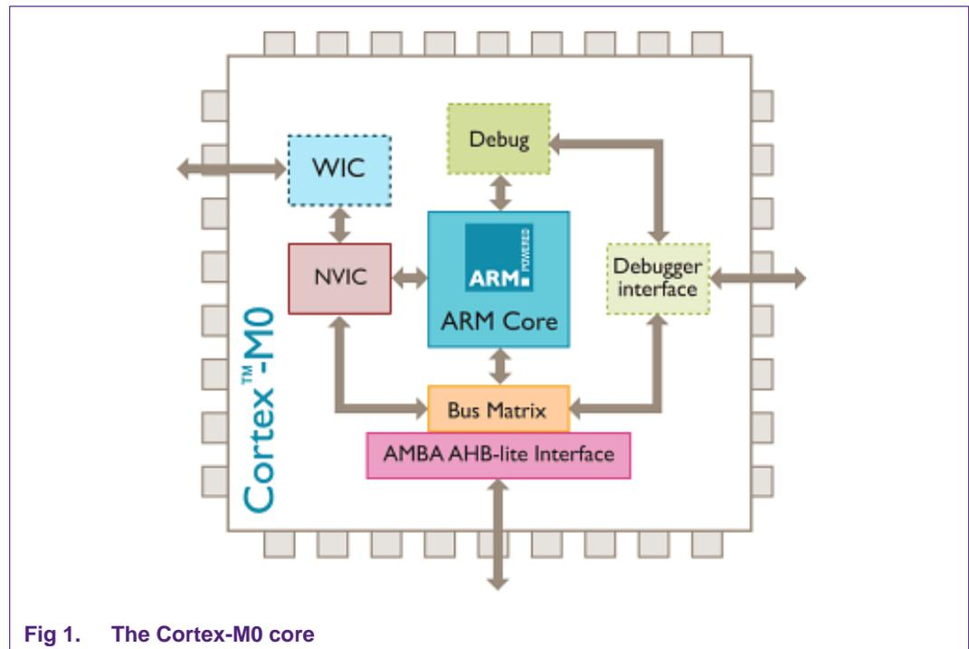
Fig 1. The Cortex-M0 core
