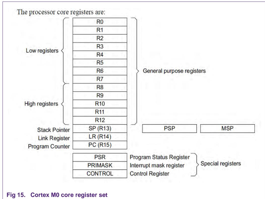
Fig 15. Cortex M0 core register set
