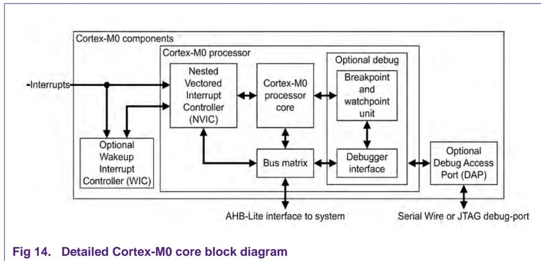
Fig 14. Detailed Cortex-M0 core block diagram
