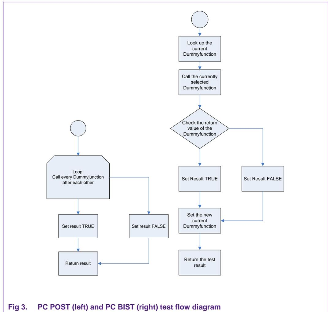
Fig 3. PC POST (left) and PC BIST (right) test flow diagram
