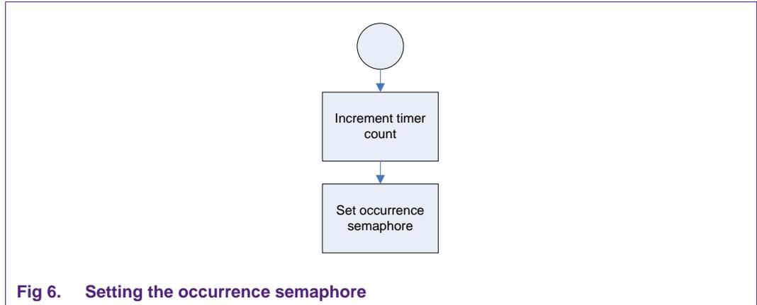
The RTC function also sets an occurrence semaphore, to be tested from the main function. Then it checks the timer counter variable to be within the estimated boundaries. The result of this check is stored into a result semaphore.
