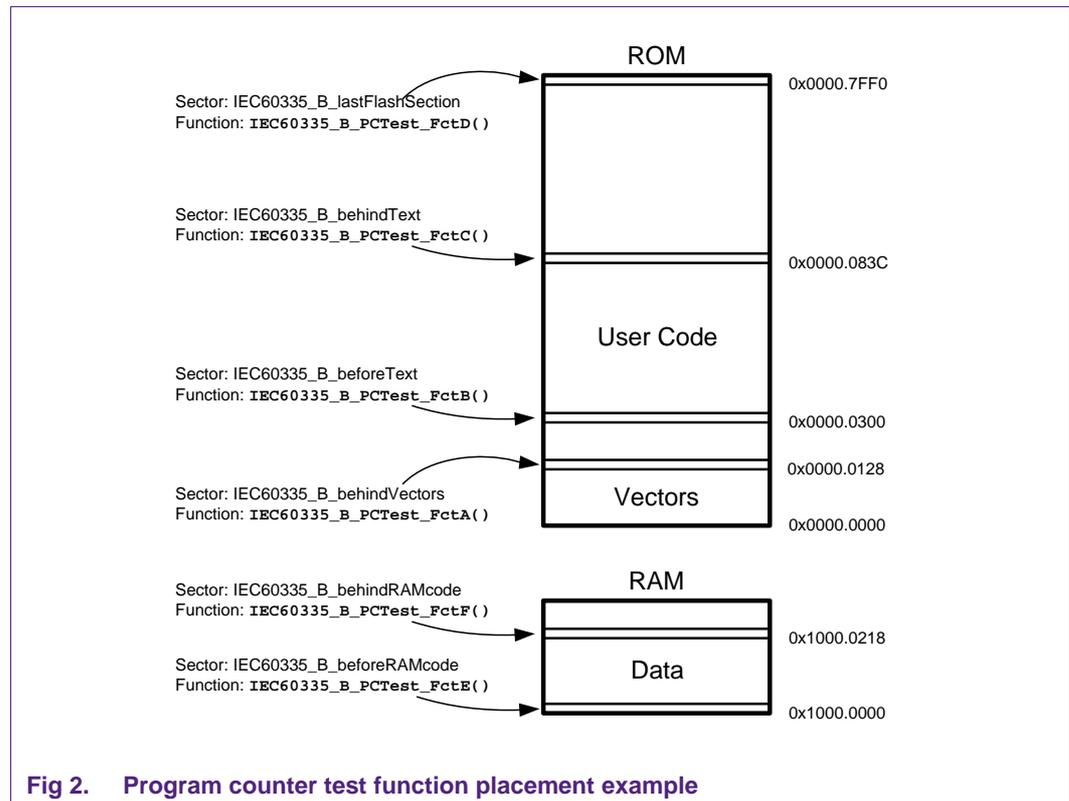
The allocation of the PC dummy test functions are placed accordingly by use of sections defined in the linker file.
