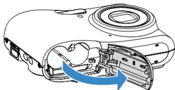
2. Insert the battery into the battery slot in the correct position as shown in the following diagram:
