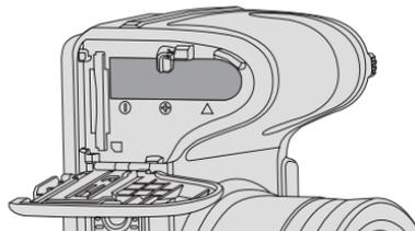
3. Insert the memory card into the memory card slot as shown in the diagram below:
