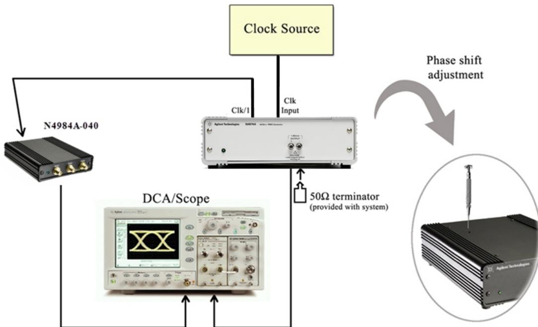
Figure 11. Re-timer phase adjustment setup
