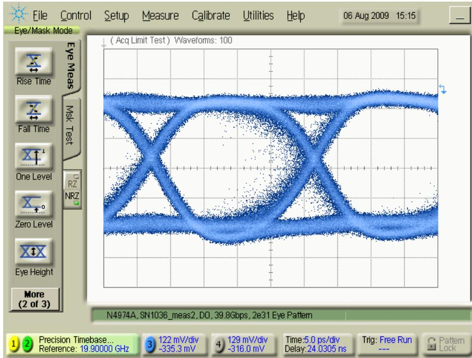
Figure 13. Eye with re-timer phase alignment almost correct
