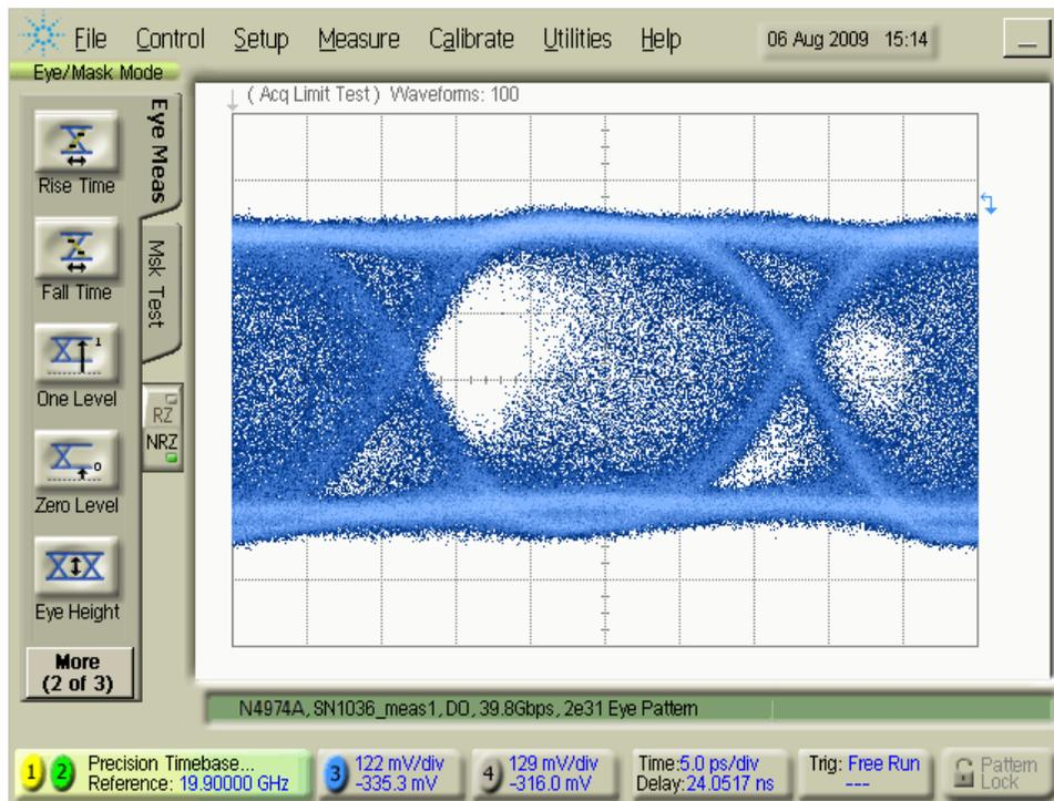
**Figure 12. Eye with re-timer out of phase alignment**
