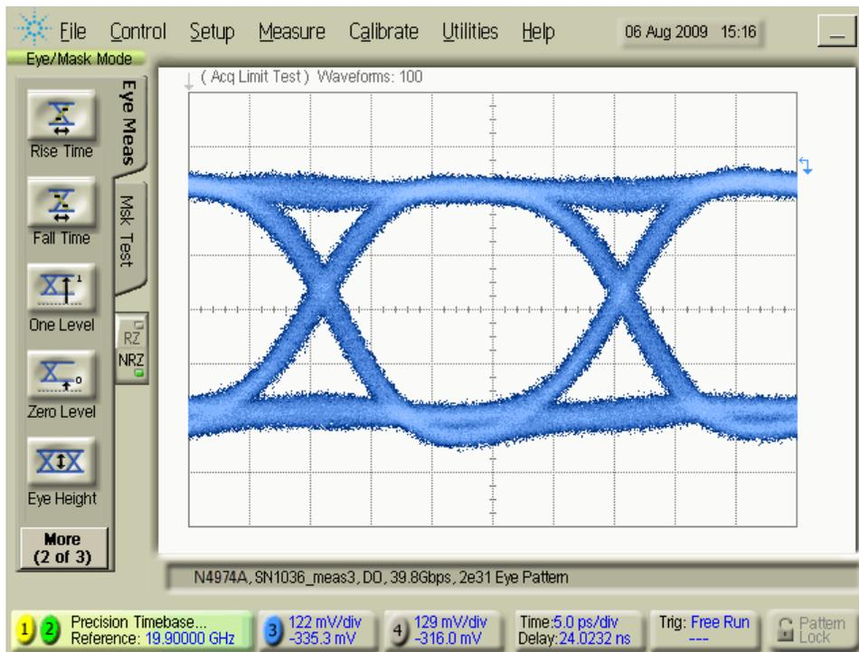
Figure 14. Eye with re-timer phase at optimum alignment
