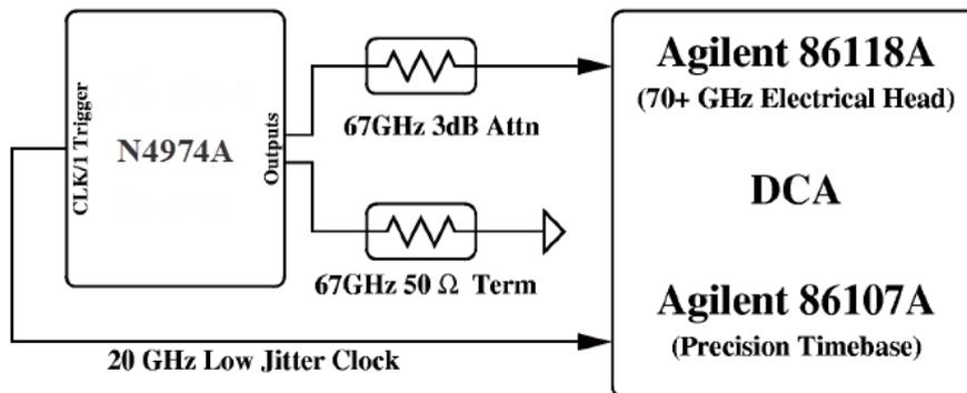
Figure 5. Verification setup
