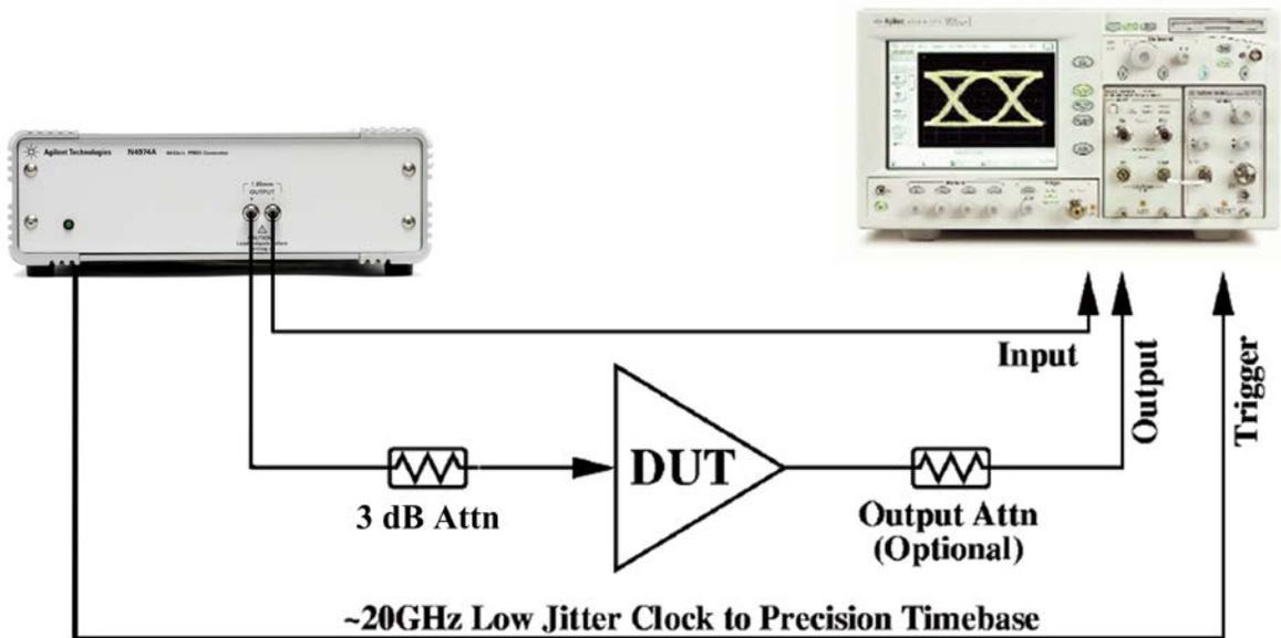
Figure 7. N4974A generic test example experimental setup
