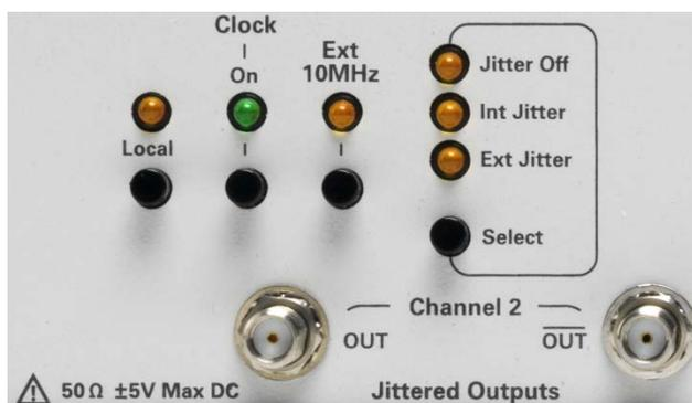
Figure 8. N4963A front panel – local, receiver, and data path controls
