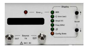
Figure 9. N4962A front panel - display panel
