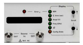
Figure 12. N4962A front panel – display selection controls
