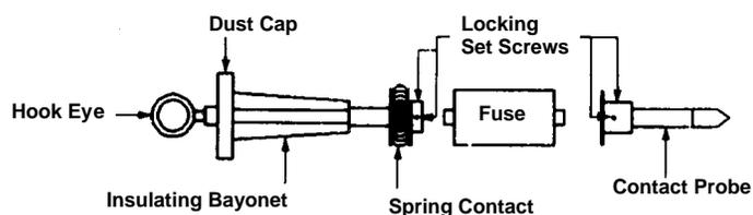
**WARNING: ASSEMBLE AND OPERATE FUSEHOLDER PER THESE INSTRUCTIONS. FAILURE TO DO SO CAN RESULT IN SEVERE INJURY, DEATH OR PROPERTY DAMAGE.**
