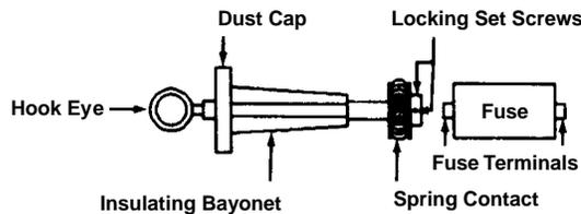
**DANGER: DE-ENERGIZE THE TRANSFORMER BEFORE REMOVING OR INSTALLING THE DEADBREAK DRAWOUT FUSEHOLDER ASSEMBLY. FAILURE TO DO SO WILL RESULT IN SEVERE INJURY, DEATH OR PROPERTY DAMAGE.**
