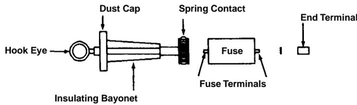
**DANGER: DE-ENERGIZE THE TRANSFORMER BEFORE REMOVING OR INSTALLING THE DEADBREAK DRAWOUT FUSEHOLDER ASSEMBLY. FAILURE TO DO SO WILL RESULT IN SEVERE INJURY, DEATH OR PROPERTY DAMAGE.**
