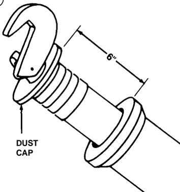
JERK THE FUSEHOLDER OUT APPROXIMATELY 6" TO OPEN THE CIRCUIT. WAIT A FEW SECONDS FOR OIL TO DRAIN BACK INTO THE TANK, THEN COMPLETELY WITHDRAW FUSEHOLDER.
