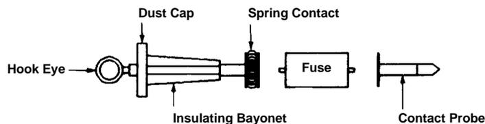
**WARNING: ASSEMBLE AND OPERATE FUSEHOLDER PER THESE INSTRUCTIONS. FAILURE TO DO SO CAN RESULT IN SEVERE INJURY, DEATH OR PROPERTY DAMAGE.**
