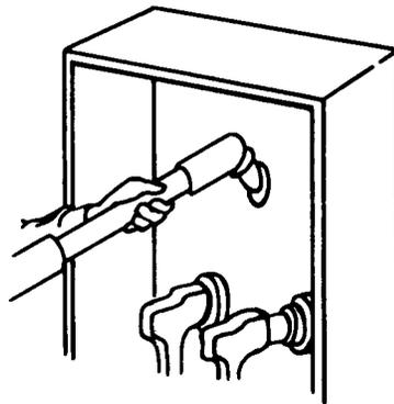
ATTACH HOT-LINE TOOL TO HANDLE EYE, STAND TO ONE SIDE AND UNLOCK THE HANDLE.
