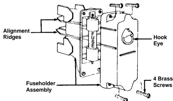
**DANGER: DO NOT ATTEMPT TO REPLACE FUSES WITHOUT FIRST WITHDRAWING THE FUSEHOLDER ASSEMBLY FROM THE HOUSING. FAILURE TO DO SO WILL RESULT IN SEVERE INJURY, DEATH OR PROPERTY DAMAGE.**
