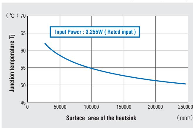
Fig 4 (b) Characteristic of input power - junction temperature  $T_j$
