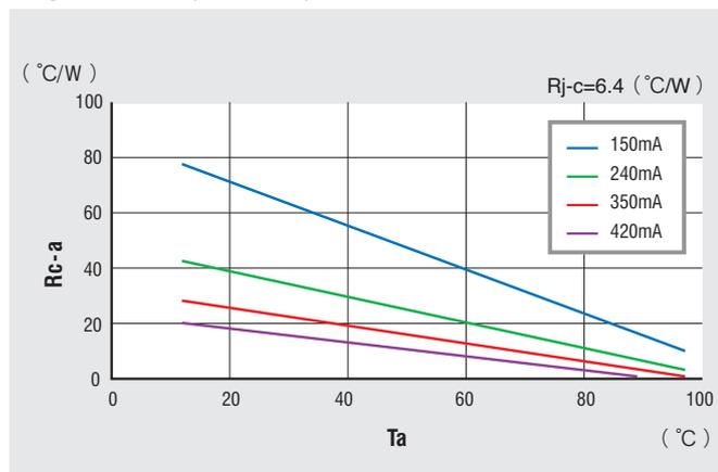
Figure-3  $T_a$ - $R_{c-a}$  ( CL-103-C6 )
