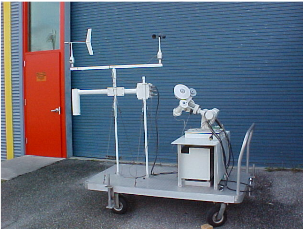
Figure 3a. Ambient cart. Pyranometer and pyroheliometer are on the right. Anemometer and wind direction indicator are on the upper left. Ambient temperature RTD, thermocouple and humidity bulk polymer sensor are in vertical canister on lower left. Oven with data acquisition modules are on lower left.
