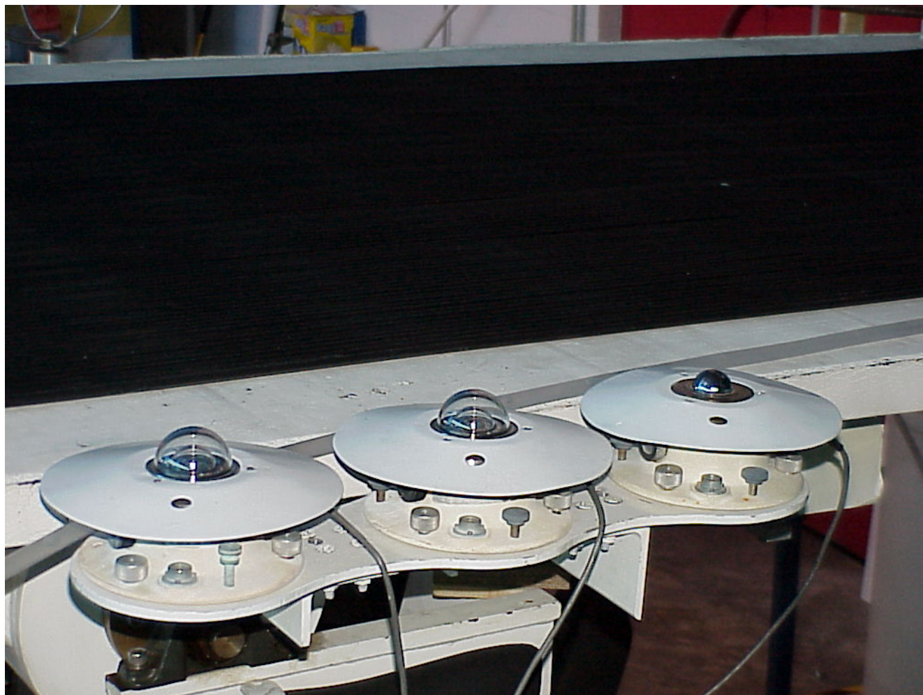
Figure 1. Pyranometers on MTP1. Primary is in the middle and secondary on the left. Pyrgeometer is on right. Flat black surface in upper background is a plastic swimming pool solar heater under test.
