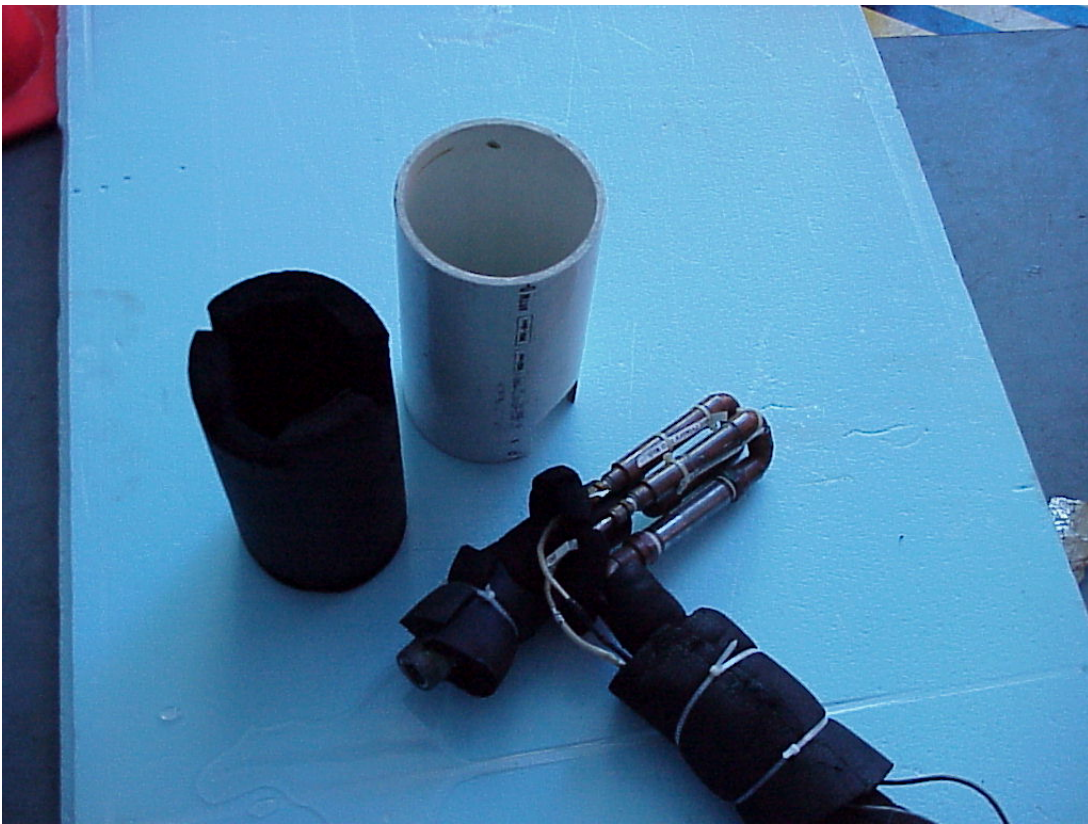
Figure 2a. General view of Inlet RTD's with insulation removed. Insulation and white PVC radiation shield are in upper part of picture.
