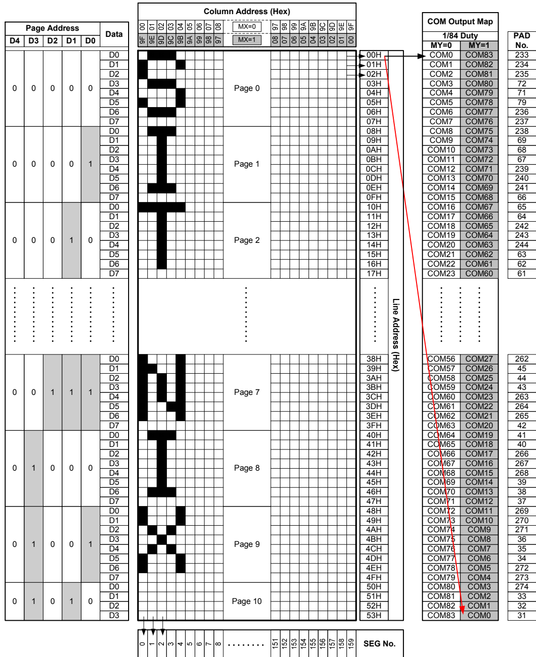
Fig 7. DDRAM and Output Map (COM/SEG)
